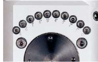
Indexing mechanism in 1° increments
