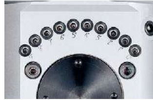
Indexing mechanism in 1° increments
