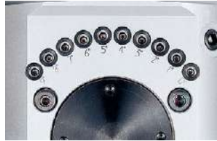
Indexing mechanism in 1° increments
